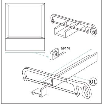
2 Install bottom guide (16) in center of bottom track (1). Then remove the bottom guide to install alass.
